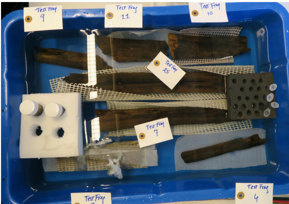
Figure 6. PEG retreatment in SO-II. For SO-III Reconservation, the large number of objects that will undergo reconservation at the same time (ca 20 objects per box) make it imperative to design a way to keep track of each one in the setup phase, so that it can be returned to its original storage box.
