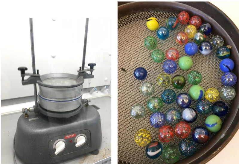
Figure 3 The Retac 3D sieving machine and the 4 mm \varnothing sieve with the 30 glass marbles.
