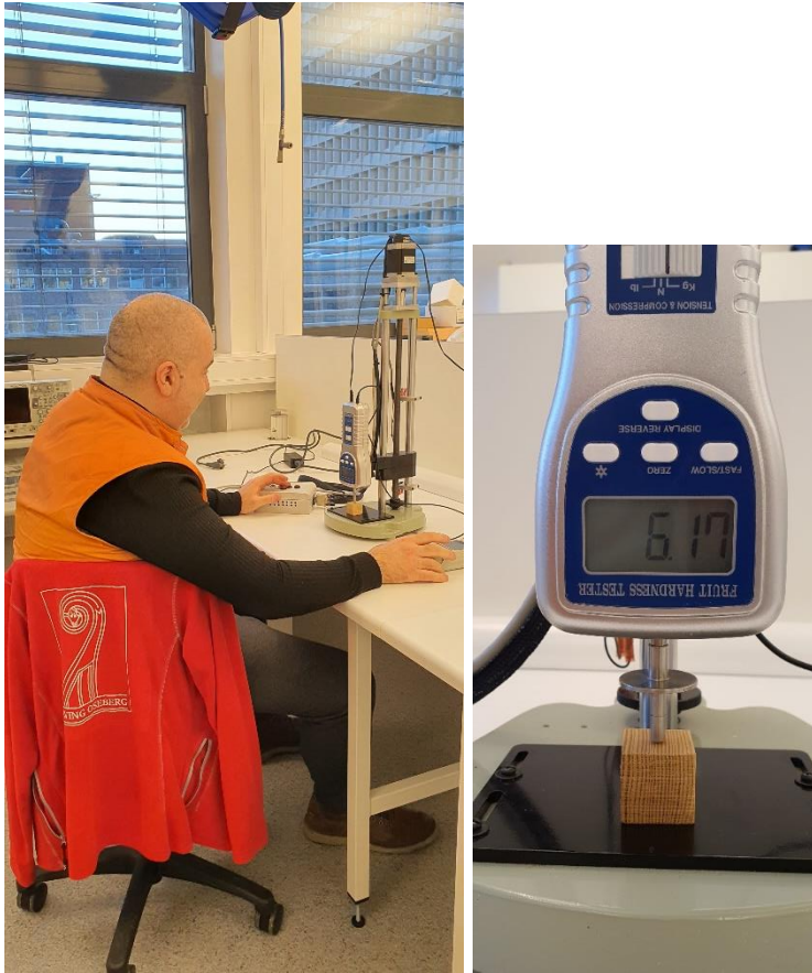
Figure 2 Testing hardness of treated wood Test Specimen using an in-house motorised commercial fruit hardness tester (with Calin Steindal).
