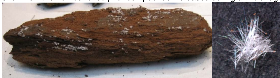
Figure 61 Fragment 1B is seen after 6 days in the climate chamber with white efflorescence on the surface, and a cluster of these crystals, approximately 1 mm across, was photographed using a stereo microscope
