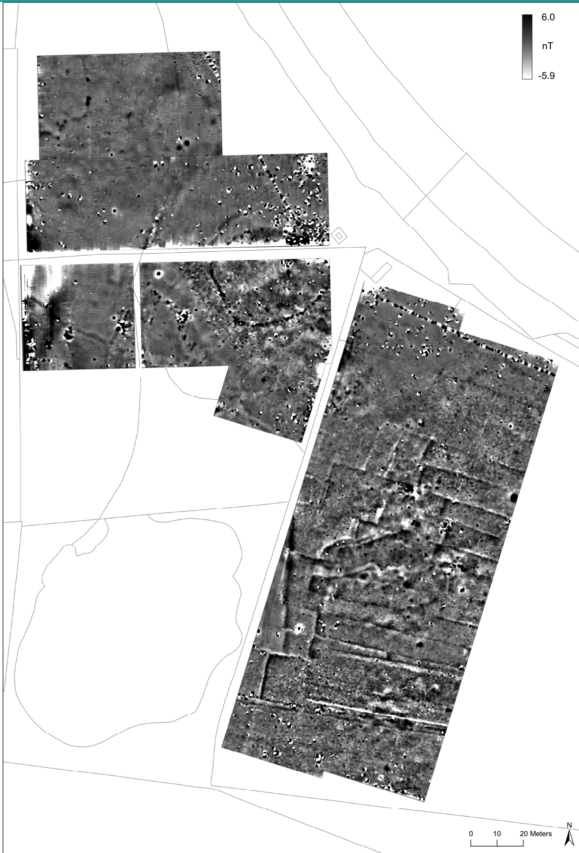
Illustration 8 Greyscale plot of the enhanced geomagnetic survey data, stretched to \pm 1 standard deviation, overlain on the O.S. cadastral map (© Crown Copyright/database right 2010. An Ordnance Survey/EDINA supplied service). Map created by Joris Coolen and Alexandra Sanmark.
