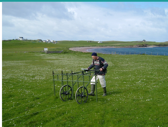
Illustration 7 The Sensys multichannel fluxgate gradiometer system in use at Housa Voe, Papa Stour (photograph by Joris Coolen).
